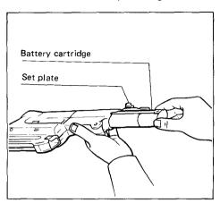
Do not use force when inserting the battery cartridge.
